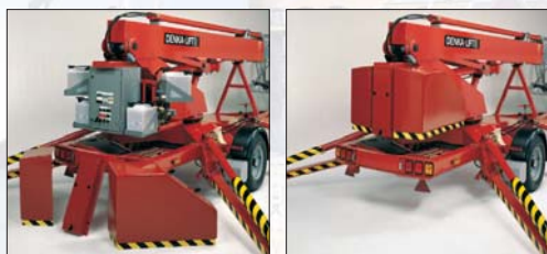
The functional design of the covering boxes for batteries, hydraulic and electric control facilitates and rationalises service and maintenance.
